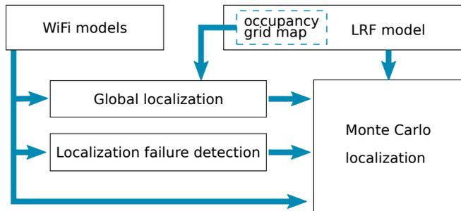
Fig. 1. Overview of our proposed approach and its two main components (i) global localization module and (ii) localization failure detection.
