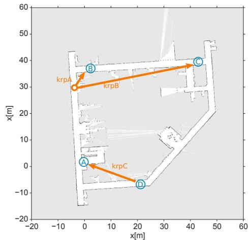
Fig. 5. Floor map of the environment where tests were performed. Locations A, B, C, and D in the environment were used as initial points for testing global localization. While paths krpA, krpB and krpC show the locations of the robot before and after each of the emulated kidnappings.
