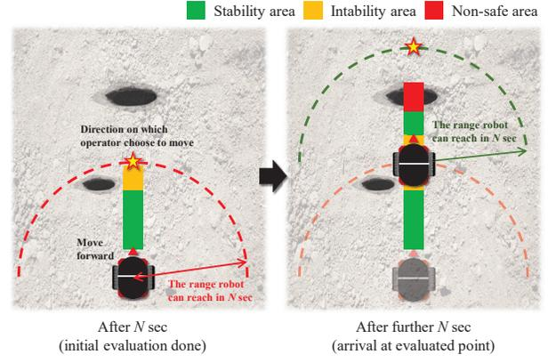
**Fig. 3:** Bird's-eye view of the schematic of the proposed visualization method.
