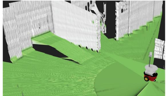
**Fig. 6:** A scene from the proposed simulator using Vortex Studio, which includes a physics engine. The physical properties of the robot such as the center of mass and inertia were set that it accurately simulates the behavior of the robot on the measured terrain.
