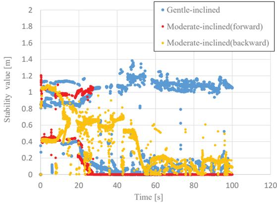
Fig. 8: Stability value when the mobile robot moved down each type of slope on the simulator. The mobile robot moved on a flat terrain for about 10 s before descending each type of slope.
