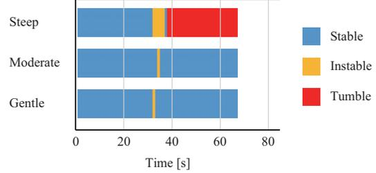
(a) Stability criterion for climbing up each type of slope on the simulator. In regard to the steep-inclined slope, the stability criterion showed that the robot would tumble
