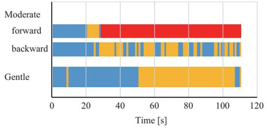
(b) Stability criterion for descending each type of slope on the simulator. In regard to the steep-inclined slope, the stability criterion was not calculated because the robot could not climb up the steep-inclined slope. Furthermore, in regard to the moderate-inclined slope, the stability criterion showed that the robot would tumble when the robot's orientation was forward. Therefore, in addition to this, the stability criterion when the robot's orientation was backward was calculated.
