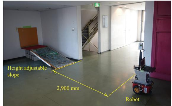
**Fig. 5:** Experimental environment: There is a slope-shaped apparatus whose angle can be adjusted. The robot scanned the environment at the position shown in this figure (at a distance of about 3,000 mm from the slope), and evaluated the safeness of the terrain.
