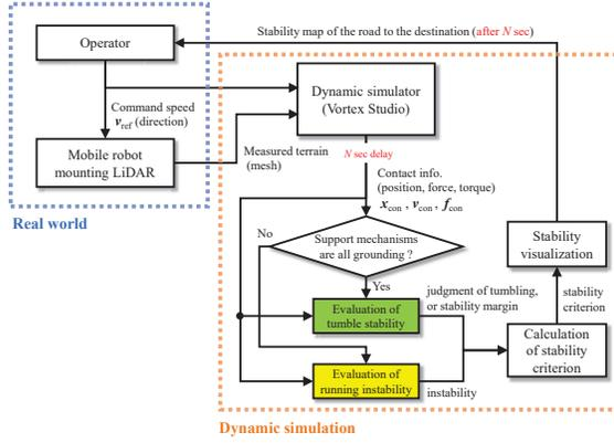
**Fig. 1:** Schematic of the proposed method. The visualized stability of the terrain to the destination is fed back to the teleoperating operator.
