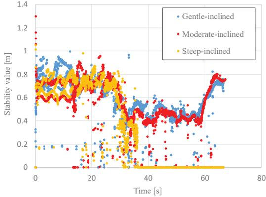
Fig. 7: Stability value when the mobile robot moved up each type of slope on the simulator. The mobile robot moved on a flat floor for about 30 s before climbing each type of slope.
