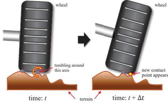
**Fig. 2:** Change of contact points after tumbling. If no contact point satisfies eq. (3) at time  $t$ , the robot is evaluated to be tumbling at the next moment. However, actually the new contact points that can support the robot will be able to appear at time  $t + \Delta t$ . Therefore, the stability of the robot should be evaluated in continuous time.
