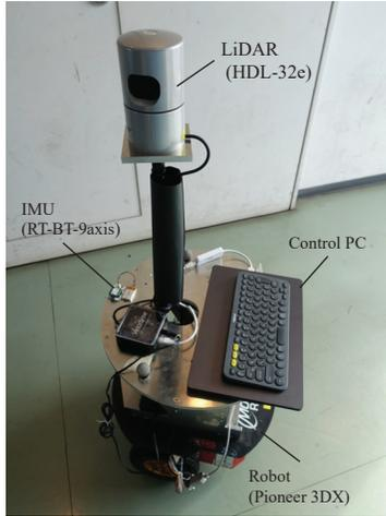
**Fig. 4:** Robot used in the experiment: Pioneer 3DX with a mounted LiDAR HDL-32e.
