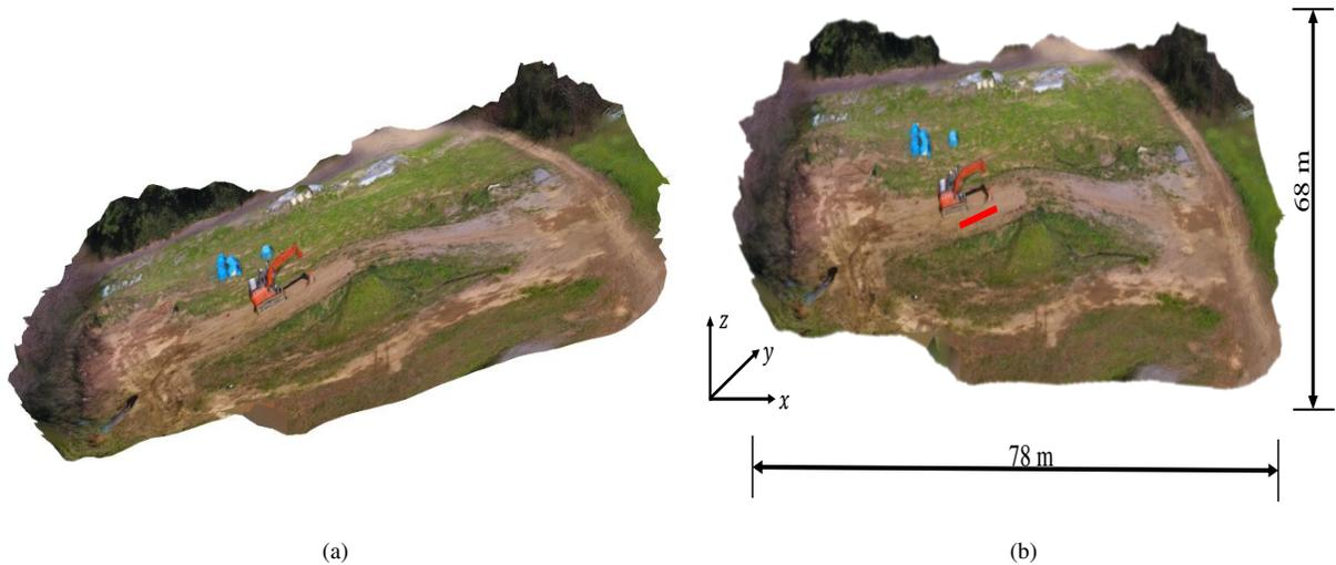
Fig. 6. Original 3D map and regenerated 3D map: (a) original 3D map built by SfM, which has no scale and slope information and (b) regenerated 3D map that has scale and slope information.
