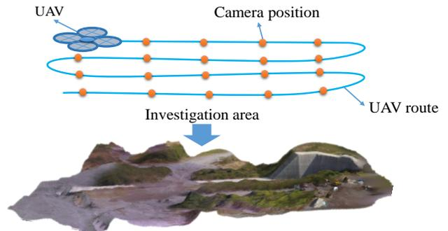
Fig. 2. 3D map generation by UAV. 3D environment can be reconstructed from 2D images taken by UAV. Blue line represents flight route and orange points represent positions of camera mounted on UAV.
