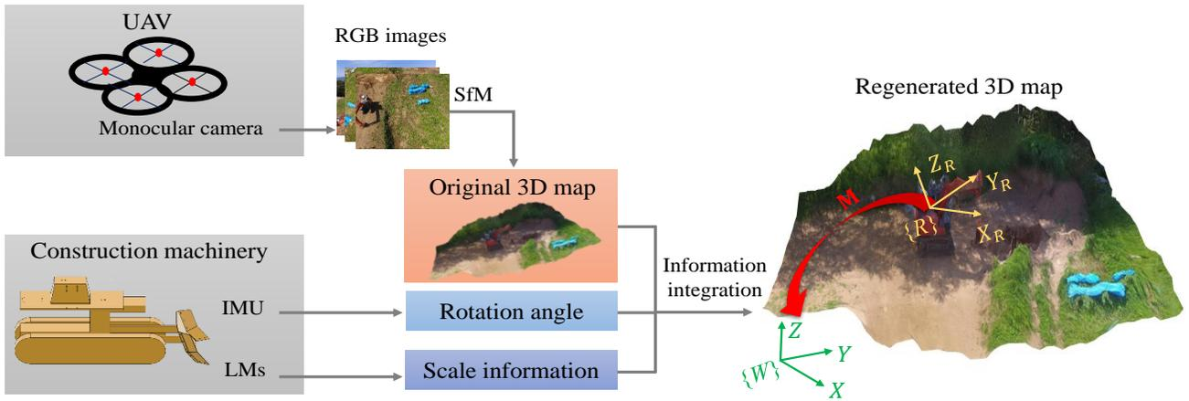
Fig. 3. Overview of proposed method. Firstly, original 3D map that has no absolute slope and scale information is generated from 2D images using SfM algorithm. Then, IMU data and marker information are used to obtain slope and scale information, respectively. Finally, 3D terrain map can be generated by integrating all of this information.
