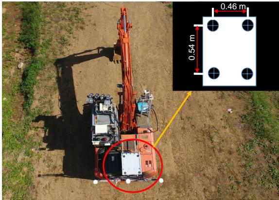
Fig. 5. Position and size of LMs attached to the construction machine. Fore LMs are attached in rectangular arrangement.
