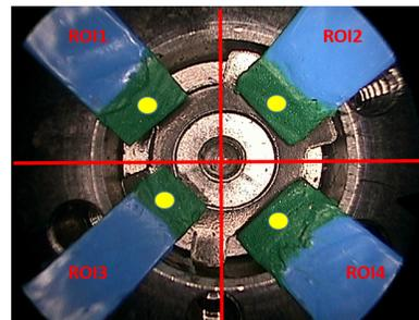
Fig. 6. Image processing algorithm: Position of the beams in the image at the maximum displacement (indentation of  $2.5\text{mm}$ ).
