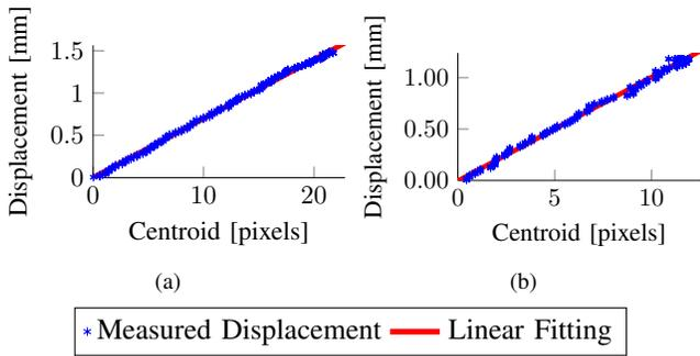
Fig. 7. Image processing algorithm: Relation between tracked feature centroid and displacement of the soft beam (a) and stiffer beam (b).
