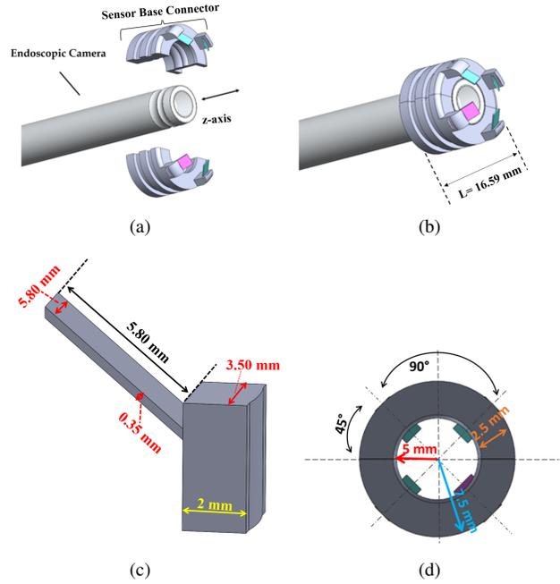
Fig. 2. CAD Drawing: (a) Exploded view of the prototype. (b) Sensor assembled at the tip of an endoscopic camera. (c) Specification of the cantilever. (d) Camera field of view.
