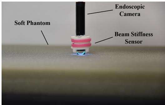
Fig. 8. Stiffness Computation of Soft Phantom: Experimental Setup.
