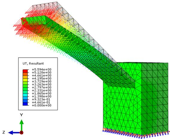
Fig. 3. FEA results showing the mesh, the boundary conditions and the displacement of the cantilever due to a normal force.
