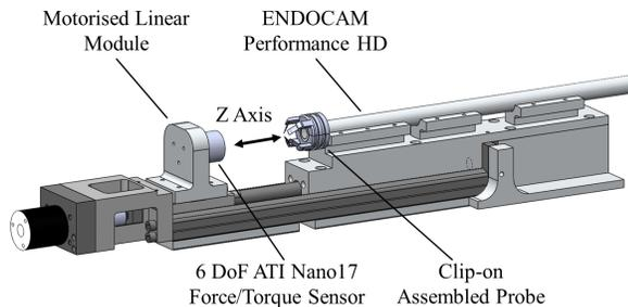
Fig. 4. Calibration device: The motorised linear module pushes the ATI Nano 17 Force/Torque sensor against the stiffness sensor whilst recording the interaction forces and the displacement.
