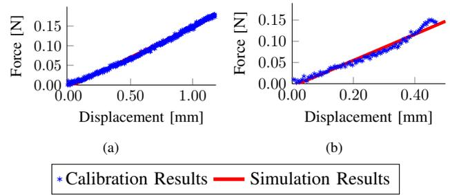
Fig. 5. Stiffness sensor for endoscopic camera: Evaluation Results. Displacements of the nitinol beams along the vertical axis in simulation and calibration of the soft beam (a) and the stiffer (b).
