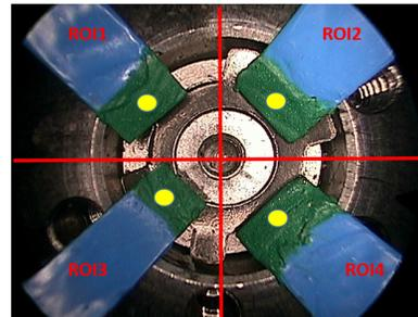
Fig. 6. Image processing algorithm: Position of the beams in the image at the maximum displacement (indentation of  $2.5mm$ ).
