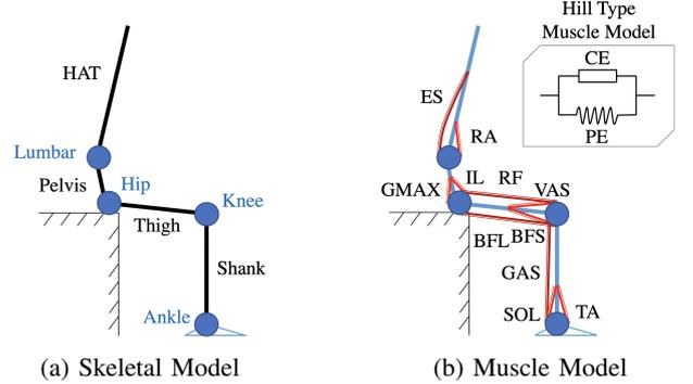
Fig. 1. Musculoskeletal model. (a) Skeletal model for joint torques calculation by inverse dynamics. (b) Hill Type muscle model for forward dynamics simulation.
