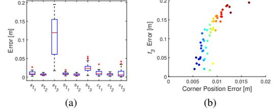
Fig. 9. Error in the case distance = 2.5 m: (a) error in  $t_1, t_2, t_3$ , where a, b, and c refer to corner only, corner+ $b_l$ , and corner+ $b_l+b_u$ , respectively; (b) relationship between  $t_3$  and corner position error. Color refers to the corner position error.
