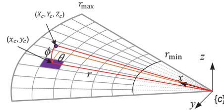
Fig. 2. Acoustic camera projection model.
