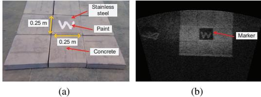
Fig. 4. Fiducial markers: (a) marker in water tank and (b) marker in acoustic image. Stainless steel with concrete offers sufficient contrast for detection.
