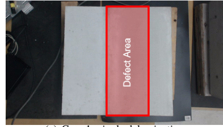
(a) Case 1: single delamination.
