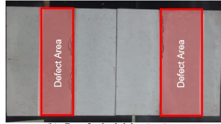
(b) Case 2: dual delaminations.
