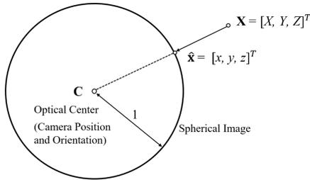
Fig. 2: Spherical camera projection model
