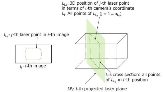
Fig. 4: The 3D laser cross section projected on the omnidirectional image captured from the spherical camera.
