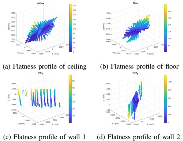
Fig. 15: Flatness of the ceiling, floor and walls. The error bar shows the distance from fitted plane.
