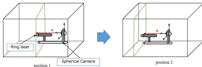
Fig. 1: The apparatus used in this research. It consists of two devices: an omnidirectional ring laser and spherical camera. By moving them around together, the images of the target environment that include the laser can be captured.
