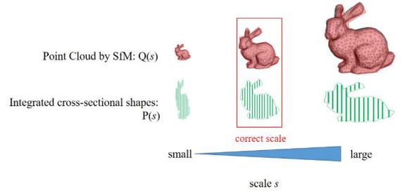
Fig. 3: Problem setting to determine the real-world scale in this research. How the shapes of the two point clouds (the SfM point cloud and the laser point cloud) change depending on the scale. When the scale  $s$  is correct one, their shapes should look the same. Using that concept, we can optimize the real-world scale  $s$  by comparing the similarity of the two point clouds.
