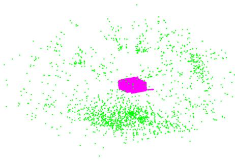
Fig. 9: The integrated cross sections of room with ground truth (pink) and SfM point cloud with scale 1 (green). It can be seen that the initial scale of SfM was far from the true scale.
