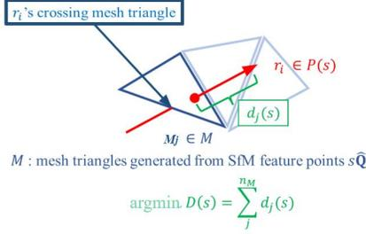
Fig. 5: Calculation of the distance between two point clouds. The SfM point cloud is converted to a mesh and its distance to the other point cloud is calculated.
