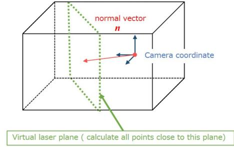
Fig. 7: Virtual Laser Plane: Since it was not possible to simulate laser illumination in Blender, a virtual cross section was used. The cross section was obtained by calculating all the points which were on a plane at a fixed distance from each camera.
