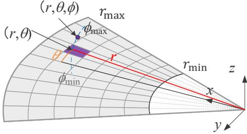
Fig. 2. Projection model. A 3D point  $(r, \theta, \phi)$  is projected to  $(r, \theta)$  in polar coordinate.
