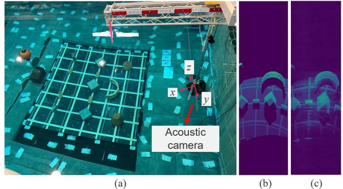
Fig. 1. Pose estimation by matching real and synthetic images. (a) Experimental environment. (b) Real acoustic image. (c) Closest synthetic acoustic image. The accurate pose of the acoustic camera can be estimated by the registration of real and synthetic acoustic images.
