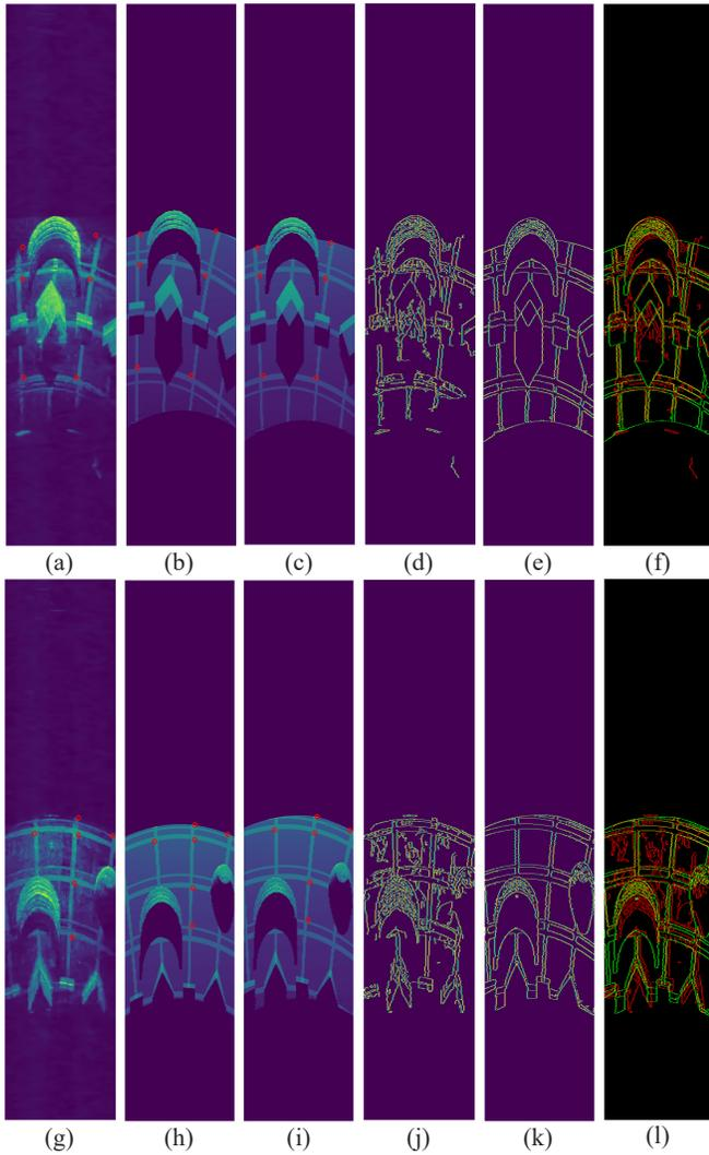
Fig. 4. Experiment results. (a) and (g) show the real images after denoising. (b) and (h) are the optimal synthetic images initial estimation. (c) and (i) are the optimal synthetic images after refinement. (d) and (j) indicate edge images from (a) and (g). (e) and (k) are the edge images from (c) and (i). We overlay (d) (e) and (j) (k) using red and green colors.
