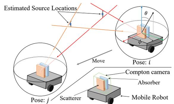
Fig. 1: Concept of the proposed method. The mobile robot stops at poses  $i$  and  $j$ . Radiation source locations are estimated as the closest points from both red and orange lines.
