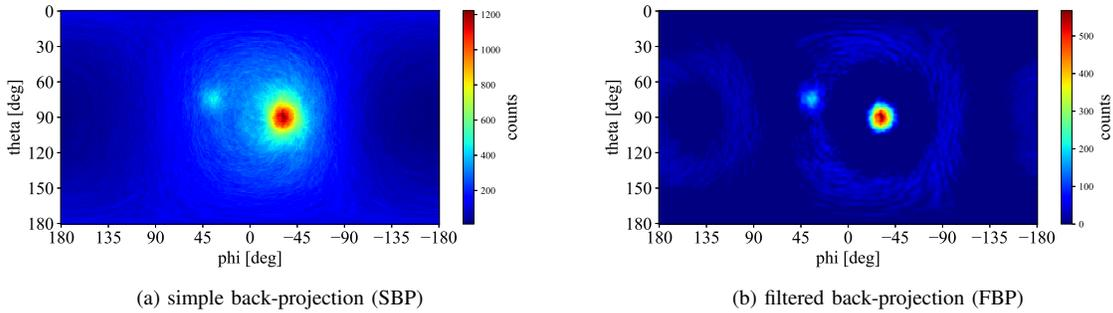
Fig. 2: The equirectangular images obtained in simple back-projection (a) and filtered back-projection (b). Points with more counts are more likely to be the source directions.
