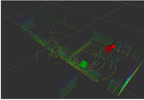
Fig. 4: SLAM and visualization of source locations. Spheres and cubes are ground truths and estimated locations by the proposed method, respectively.
