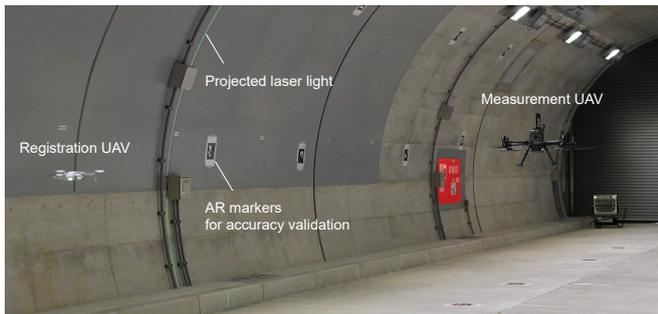
Fig. 6. Measurement conditions.
