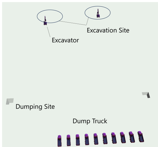
Fig. 5. Simulated environment for two teams of construction robots. At the beginning of the simulation, all robots are aligned in the waiting area on the lower side of the figure.
