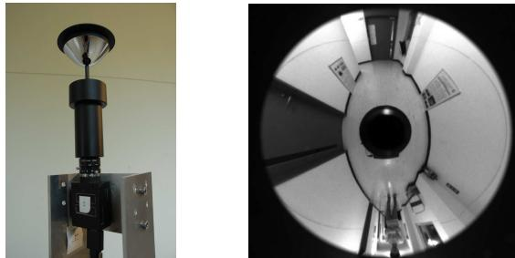
**Fig. 1.** Omnidirectional camera and acquired image.
