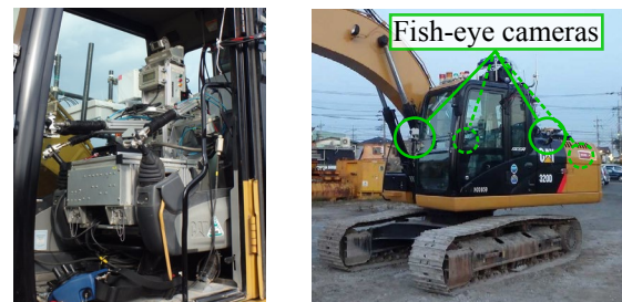
(a) Installed Robo Q (3) (b) Installed cameras
