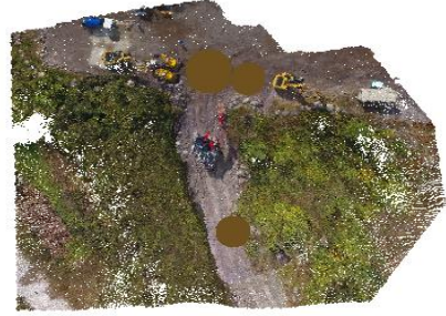
Fig. 4: The result of precise registration. Precise registration of the partial 3D terrain model and the local 3D terrain model is performed based on PFH
