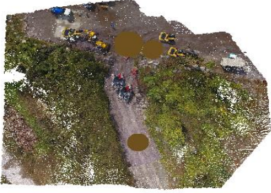
Fig. 3: The result of coarse registration. Coarse registration of the partial 3D terrain model and the local 3D terrain model is performed based on FPFH
