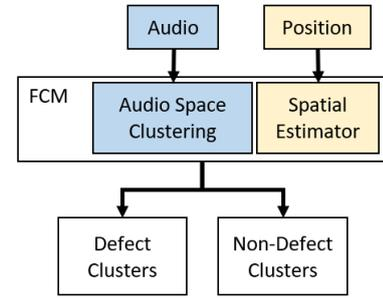
Fig. 1: FCM with Spatial estimator for defect diagnosis.
