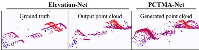
Fig. 2. Comparing the ground truth and the point cloud, transformed by the Elevation-Net, with the generated point cloud by the PCTMA-Model. The scene, captured by the sonar sensor, contains 18 objects but has a deactivated floor.
