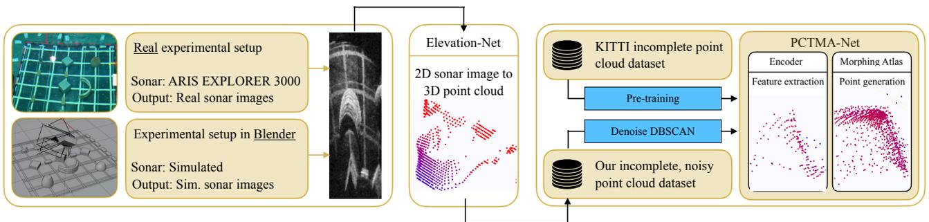
Fig. 1. Pipeline showing dataset generation in Blender, transformation of 2D sonar images into 3D point clouds, denoising of point clouds, and their completion and refinement using PCTMA-Net
