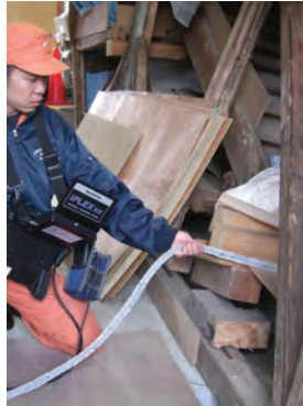
Fig. 10. Experiments of Active Scope Camera at Collapsed House Simulation Facility of IRS Kobe Laboratory.
