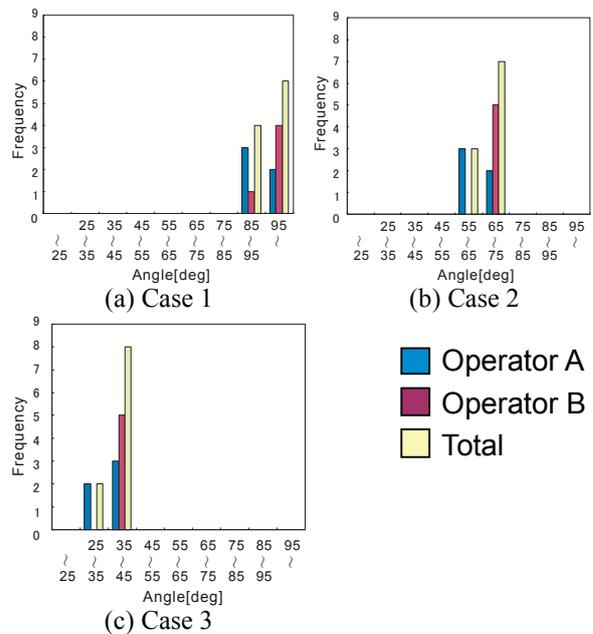
Fig. 6 Angle between bucket bottom and ground at excavation start (frequency distribution)
