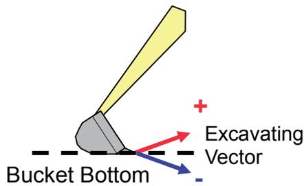
Fig. 10 Angle between bucket bottom and excavating vector
