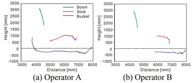
Fig. 7 Excavation trajectory of case 1
