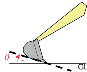
Fig. 5 Angle between bucket bottom and ground
