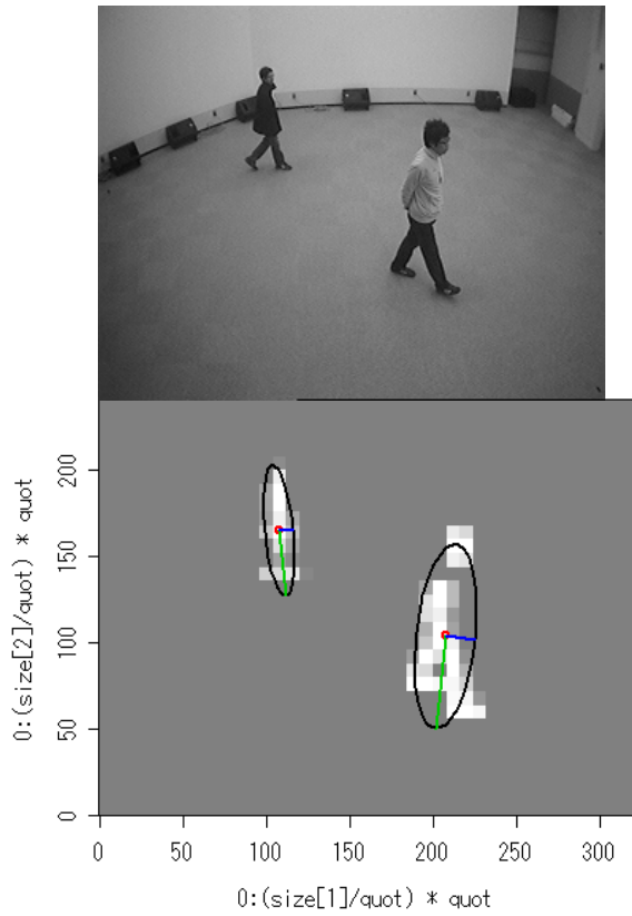
Fig. 11 Original image (upper) and image of extracting moving object process (lower)
