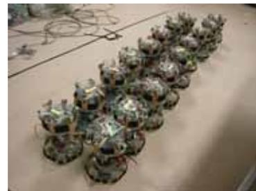
Fig. 8. Modular robot system “Slimebot”
