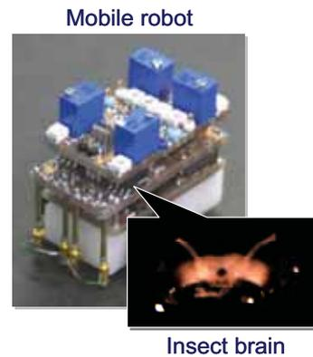
Fig. 7. Mobile robot integrated with silk moth brain
