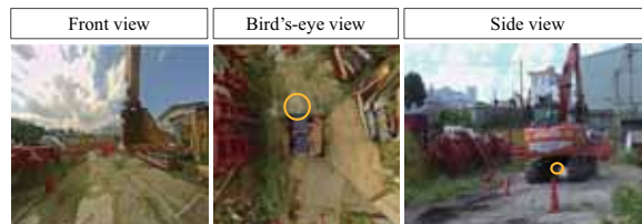
Fig. 12 Example images in controlling stop position experiment. Yellow circles indicate stop marks. Bird's-eye view can show a backhoe and a stop mark relatively.
