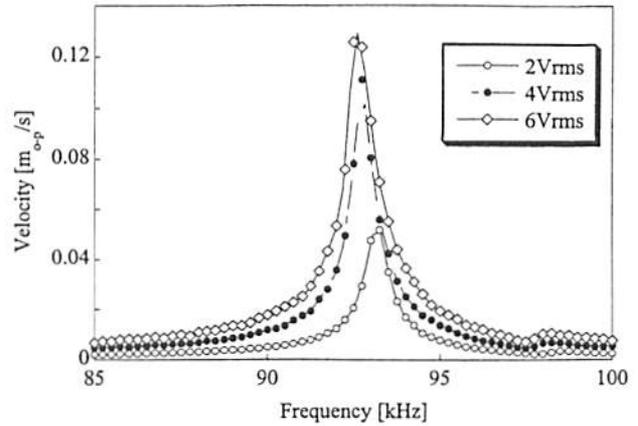
Fig. 4. Relationship between driving frequency and velocity for various input voltages.
