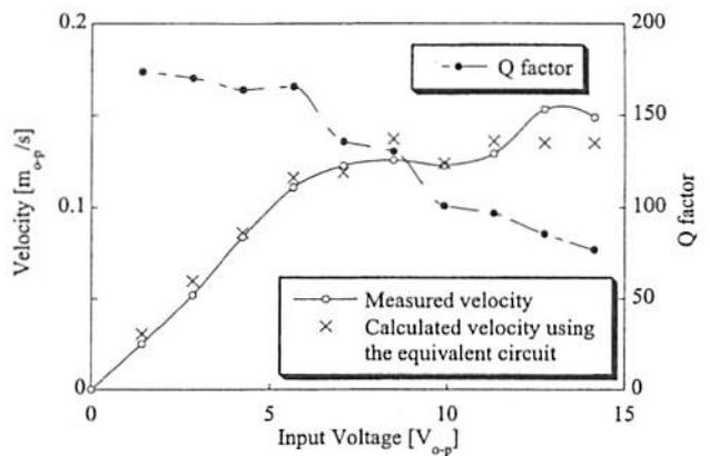
Fig. 5. Relationship between driving voltage, velocity and quality factor. Calculated data using an equivalent circuit is also given.
