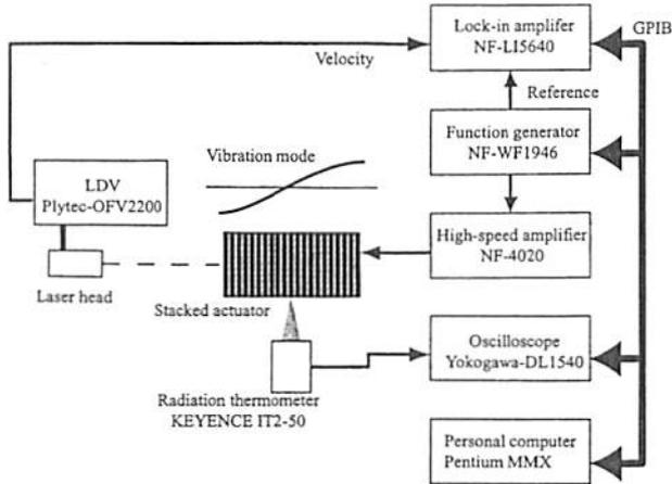
Fig. 3. Setup to measure the vibration velocity and temperature.
