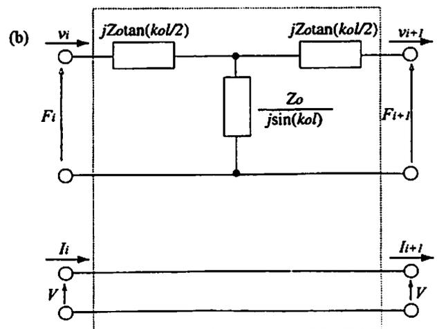
Fig. A-1. Modified Mason's equivalent circuits for piezoelectric layer (a) and no piezoelectric layer (b).
