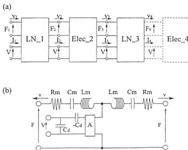
Fig. 2. Modified Mason's equivalent circuit in series (a) and a general equivalent circuit for piezoelectric transducer (b).
