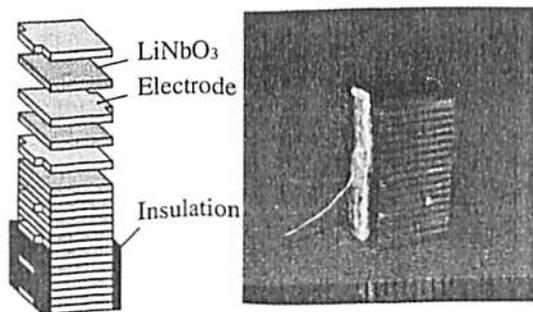
Fig. 1. Stacked actuator using lithium niobate.
