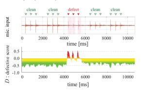
Fig. 1 The top chart shows hammering sound of time domain, and the bottom one shows the defective score *D* estimated by the proposed detector (eq. (2)).
