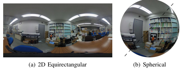
Fig. 1. Spherical Images encode information from all directions and can be represented in the (a) 2D Equirectangular and (b) Spherical Projection.
