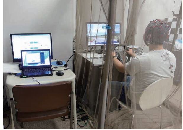
Figure 2. Experiment setup. CarSim and MATLAB was run on the laptop. The participant and the desk with driver's screen, Logitech G920 and g.USBamp were surrounded by an electromagnetic shield.
