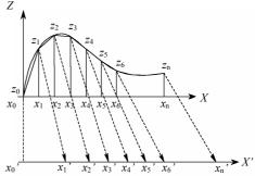
Figure 3. Geometric distortion correction.
