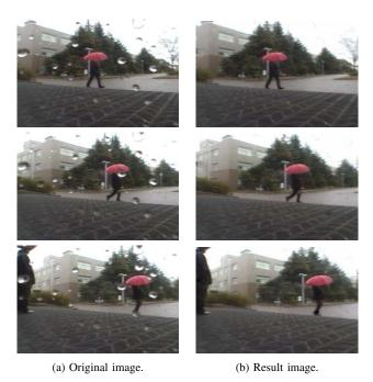
Fig. 10. Results of noise removal (waterdrop).
