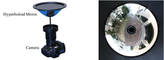
Fig. 1. The omnidirectional camera which we use is shown in the left figure. The camera attaches a hyperboloid mirror on the front of the camera lens. An omnidirectional image is shown in the right figure. The image has a 360-degree horizontal field of view.
