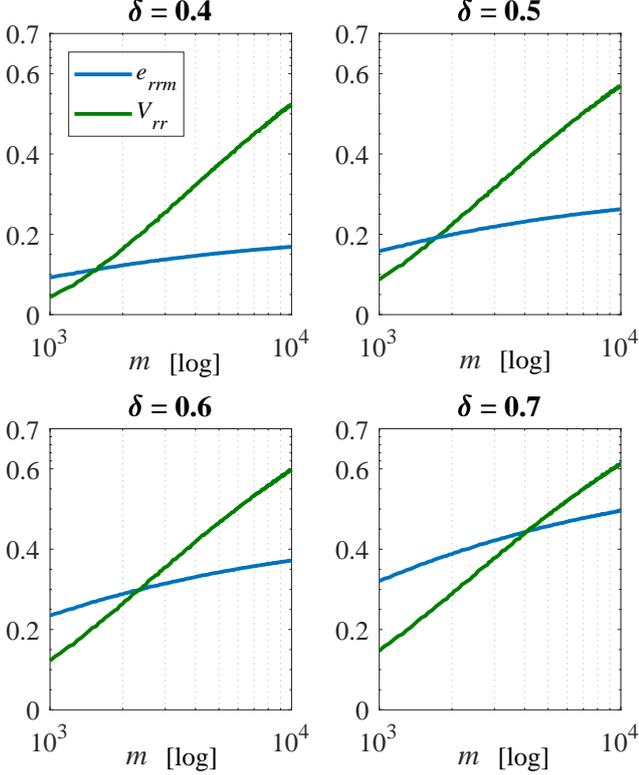
Fig. 5. For different values of  $\delta$  (the ratio between noise and signal standard deviations), two significant data are here reported as function of the observation matrix length  $m$  (in log scale). With solid blue lines, the residual relative mean error of the particles  $e_{rrm}$ . With green lines the ratio  $V_{rr}$  between the volume enclosing the particles set at the end of the PRF identification ( $V_{sol}$ ) and the volume of the total simplex ( $V_{tot}$ )
