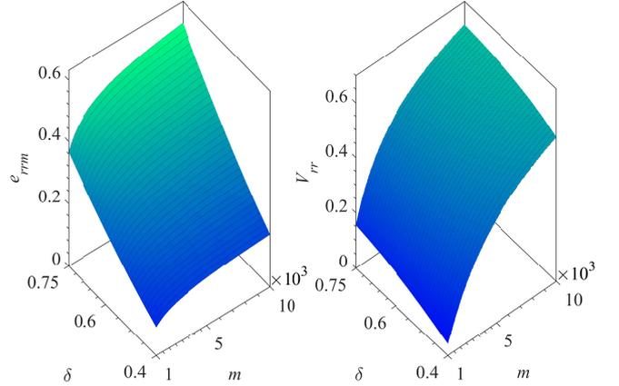
Fig. 4. As function of  $\delta$  and  $m$ , respectively the ratio between noise and signal standard deviations and the length of the observation matrix, two quantities are represented. On the left, the residual relative mean error of the particles  $e_{rrm}$ . On the right, the ratio  $V_{rr}$  between the volume enclosing the particles set at the end of the PRF identification ( $V_{sol}$ ) and the volume of the total simplex ( $V_{tot}$ )
