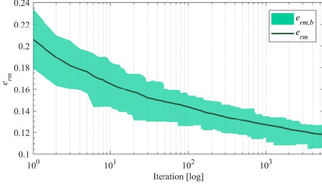
Fig. 2. Time evolution of relative mean error  $e_{rm}$  for  $m = 2000$ ,  $\tilde{\sigma}_1^2 = \tilde{\sigma}_2^2 = \tilde{\sigma}_3^2 = 0.16$  and  $\tilde{\sigma}_4^2 = 1.23$ . The solid line is the average of the values obtained in different Monte Carlo runs while the colored area ( $e_{rm,b}$ ) is enclosed by the absolute minimum and maximum values of  $e_{rm}$  in the Monte Carlo runs
