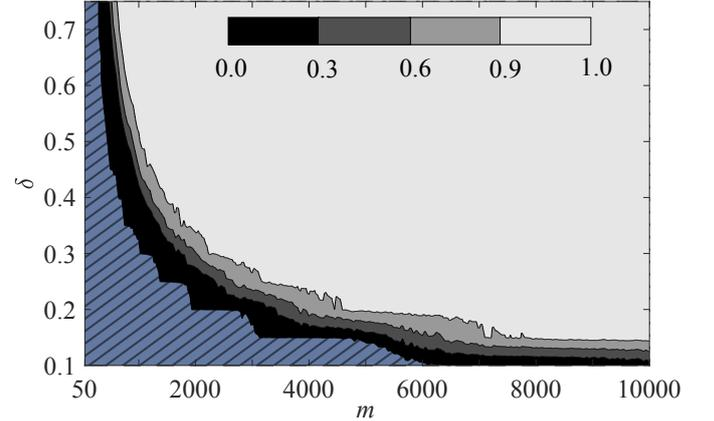
Fig. 6. Robustness map of the PRF scheme as function of  $m$  and  $\delta$ . The blue area represents the unfeasible points where the algorithm failed in at least one Monte Carlo run. The gray-scale plot represents the probability of having the true parameters vector lying inside the convex hull enclosing the “survived” particles for different Monte Carlo runs
