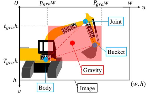
Fig. 5. Backhoe presentation position in gravity method
