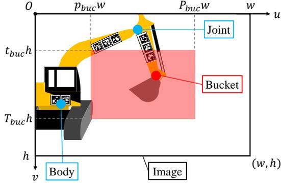
Fig. 4. Backhoe presentation position in bucket center method
