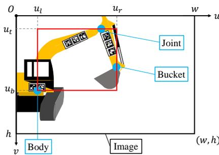
Fig. 3. Backhoe presentation position in proposed method
