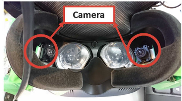
Figure 4. Two cameras installed inside the head-mounted display
