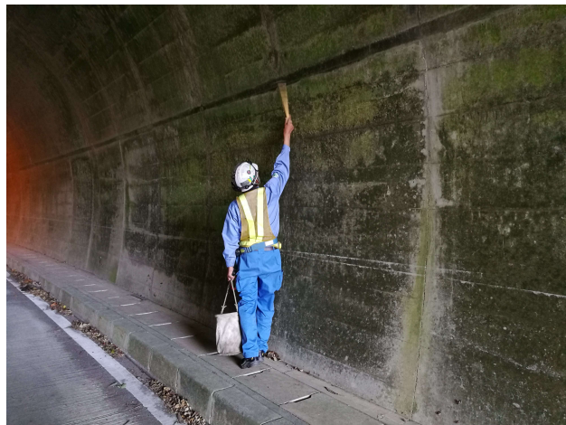
Fig. 1. Hammering test by a human inspector
