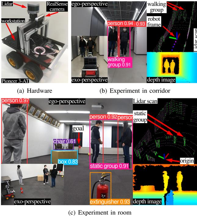
Fig. 6. Real-world experiments. (a) is the experiment hardware. (b) and (c) show snapshots of real-time experiments pictured from the robot ego- and exo- perspectives, 3D Lidar data, and depth images.
