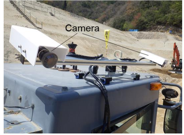
(b) Stereo camera on vibration roller
