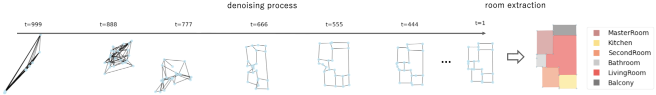
Figure 1: From a beta-noised graph to a structured floorplan, then rendered as layouts.
