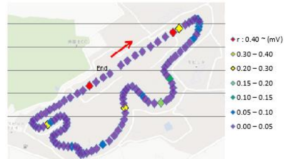
Fig. 1: Masseter muscle's RMS value (r) – car position relationship on 3rd round
