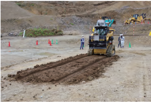
Fig.2: Trafficability judgement based on underground information [5]
