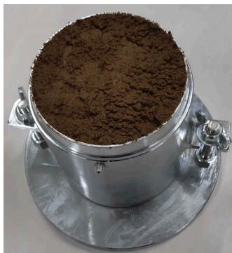
Fig.4 Soil compacted in the mould
