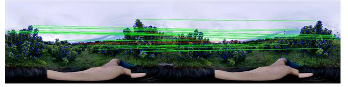
Fig.7 Feature point matching on farm using SuperPoint, k-nearest neighbor matching, and Lowe's ratio test.
