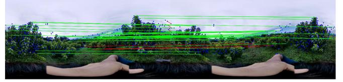
Fig.9 Feature point matching on farm using tangent plane projection, SuperPoint, mutual nearest neighbor matching, and Lowe's ratio test.
